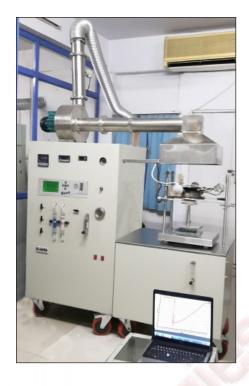
The is used for the determination of the fire behavior of the various samples in the solid state. This Device is used to collect information of the various parameters associated with the burning characteristics such as ignition time, mass loss, combustion products, heat release rate etc. of various samples. For the determination of Heat Release Rate, the Samples are exposed to the irradiative heat flux at the surface.
